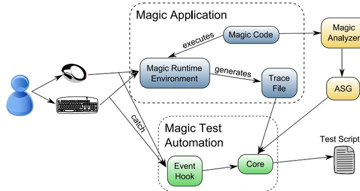
Figure 5: Recording GUI Events.
